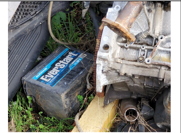
Photo 18: Lead acid battery not managed as universal waste and, therefore, is hazardous waste not managed in accordance with 40 CFR 262.
